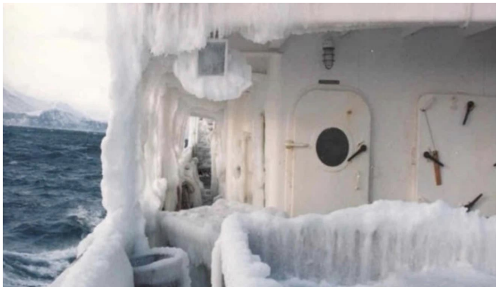
Frozen sea spray creates heavy ice buildup on vessels that can rapidly destabilize the ship, jam critical equipment, and cause capsizing.
