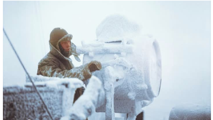
Frozen sea spray creates heavy ice buildup on vessels that can rapidly destabilize the ship, jam critical equipment, and cause capsizing.
